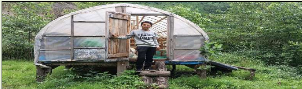
A prototype Solar Dryer made of local / recycled Materials
